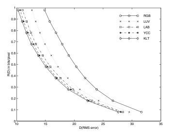
Figure 2. Rate-Distortion curve for the test image "Miniflow"
